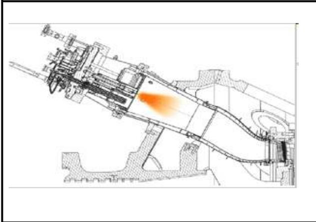
**Cross-Section of Gas Turbine Combustor**
