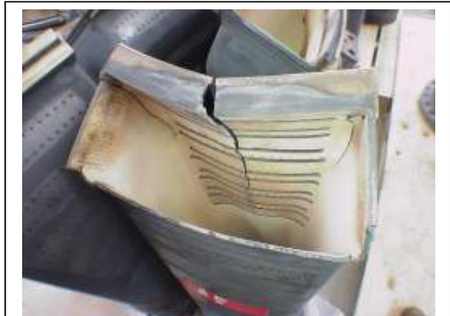
**Fractured Transition Piece Resulting from Abnormal Combustion Dynamics**
