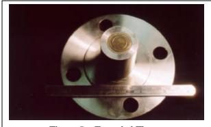
Figure 5 – Extended Flange Pressure Transducer
